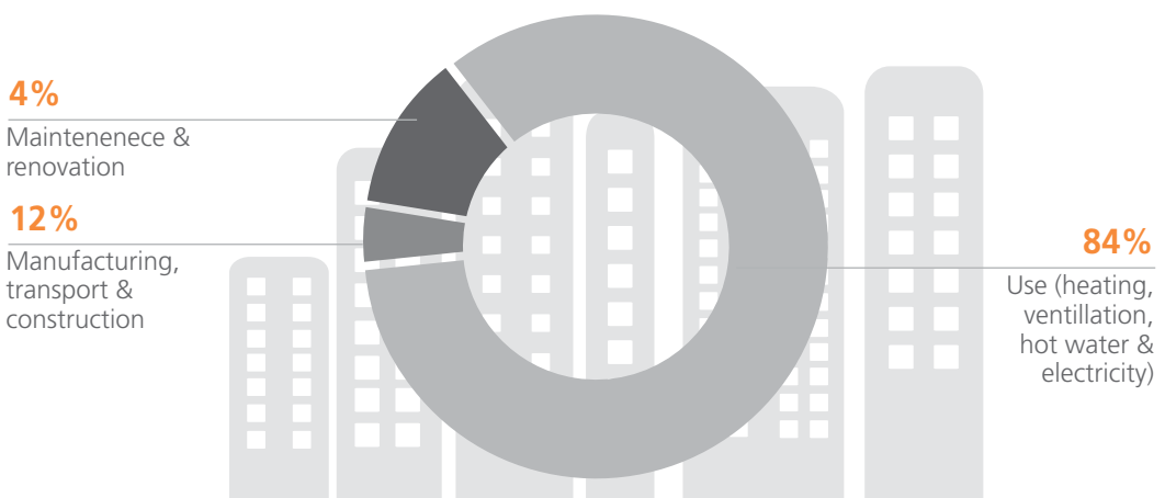
Figure 1.17 Life Cycle Energy Use of Buildings
